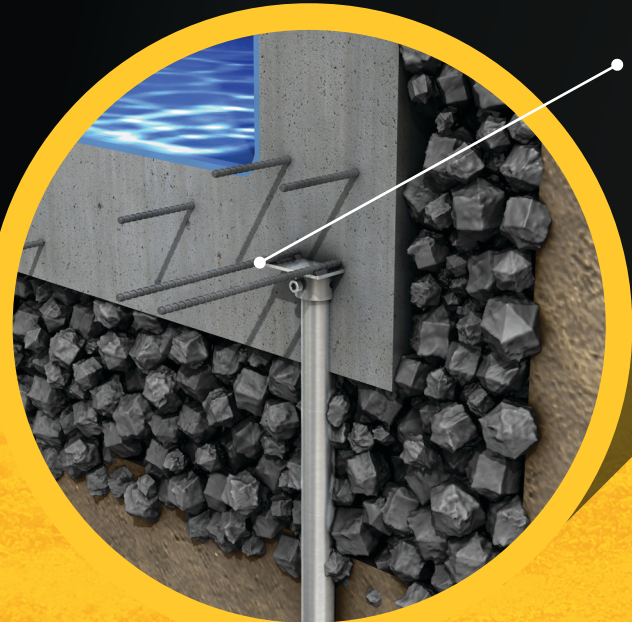
PILE HEAD WITH REBAR
